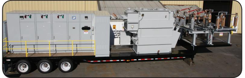
Elgin Power Solutions builds size range up to 138kV / 60 MVA systems. Our mobile substations are configured to maximize maneuverability and comply with DOT regulations.
